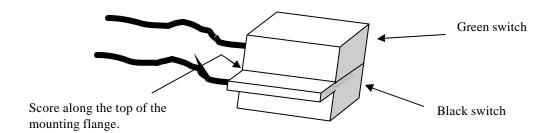
2. Once the black switch is scored across the flange top, use <u>pliers</u> to bend the outside of the flange downward then lift it back up to break it loose. The result will be a black switch that is the same width as the original green switch. The length is slightly longer however this will not hinder the switch mounting or operation.
