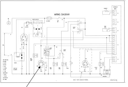
New pump capacitor (4A2128-05)
