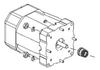
4. Re-assemble the pump assembly in reverse order assuring that the hosing is in the original position. Install the pump and check for water leaks.
