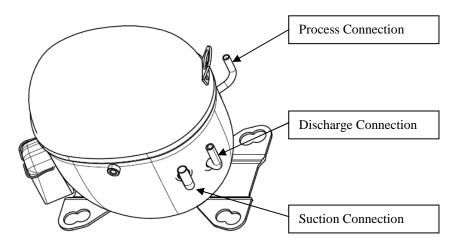
**Important:** When this compressor is used KM series unit a control board adjustment is recommended. Adjust DIP switches number 1 and 2 be moved to the "ON" position.
