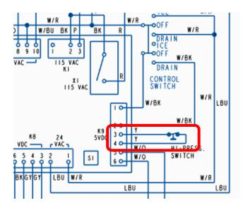
New Wiring: Pins 3&4 5V DC with new relay added
