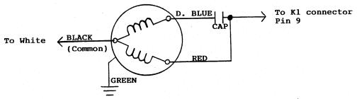
This diagram applies to all dual outlet pump motor assemblies as listed below.
