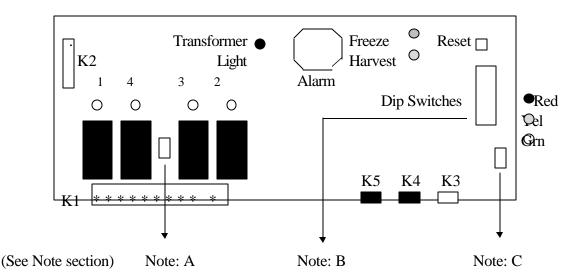
The red transformer light is illuminated to indicate that correct control voltage power is being supplied to the board through the K2 connector. If the voltage drops below 9.5 volts or rises above 14.5 volts the transformer light will de-energize and an audible alarm will sound indicating a voltage supply problem. There is an acknowledgment beep that occurs when the initial power is supplied and when power is turned OFF.
